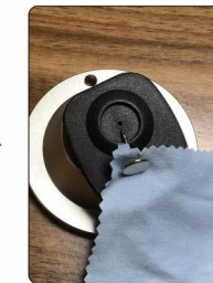
3. Remove the pin from the tag part of the detacher
